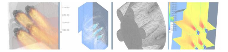
CFD ensures proper distribution of combustion air through complex geometry air duct and wind box.
