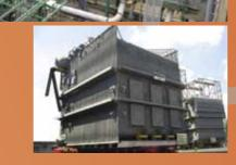
boiler model suitable for units of medium-large capacity steam capacity up to 1,100,000 lb/h steam operating pressure up to 1,600 psig steam operating temperature up to 970° F gas, oil & crude oil fired
